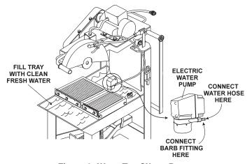
Figure 6. Water Tray/Water Pump
